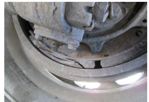
Cracked lining. OOSC, Part II, a.(5)(c)iii / 393.47(a)-U.S.
