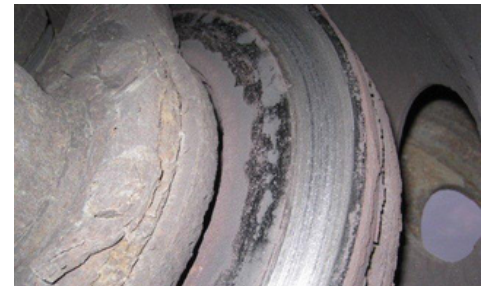
Metal-to-metal contact. OOSC, Part II, a.(6)(c) / 393.48(a)-U.S.
